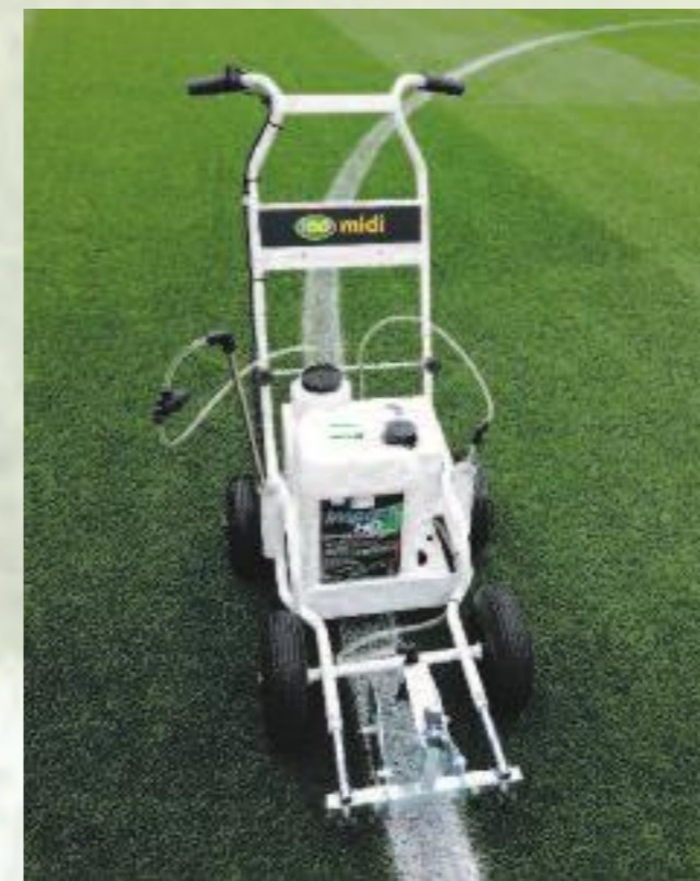
Twin probe paint circulating system for internal paint dispersion
