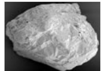
Electron micrograph of sand grain having been treated with Breaker Curative 2
