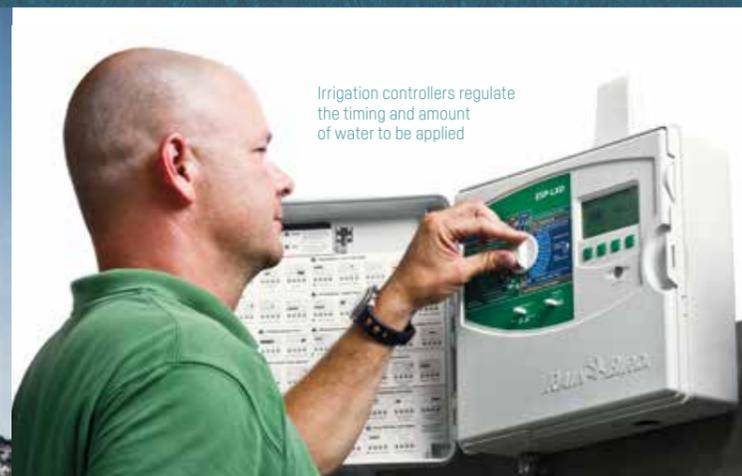
Irrigation controllers regulate the timing and amount of water to be applied
