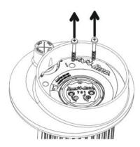
4 Align the adjustment ports on sod cup with the adjustment screws on rotor.
