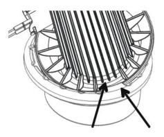
2 Press flange cover onto case flange working from wide tab towards valve switch, until flange cover snaps into place.
