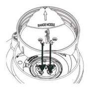
**5** Place sod cup on top of rotor and secure with screws.
