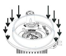
**3** Using a Phillips head screw driver remove screws from top of rotor.
