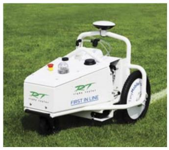
Specially developed robotic line marker for the multiple pitch marking use, contractors, service providers and extensive multisports facilities.
