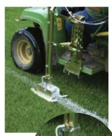
\* Locking, retractable arm for ease of operation and transportation
