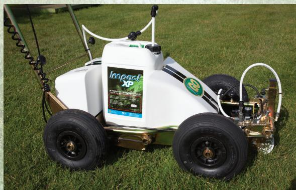
Carrying 3 x 5 litre Eco-Bags, 13 pitches could be over-marked, or using 2 x 10 litre drums up to 18 pitches can be over-marked, without returning to base or carrying a heavy tank of dilutable paint and water which can cause compaction on wet, winter pitches.
