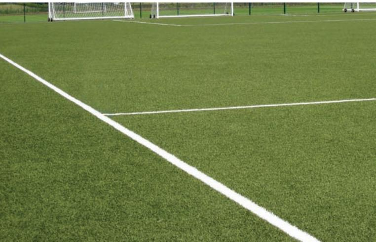
The paint has superior drying qualities and under dry conditions in moderate temperatures above 5°C will become rainfast in as little as 20 minutes.
